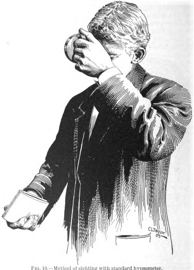
FIG. 10.—Method of sighting with standard hypsometer.
